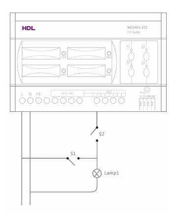
Turn on Lamp1: Turn on S1, doesn't matter the S2 is on or off. Turn off Lamp1: Turn off S1 and S2.
