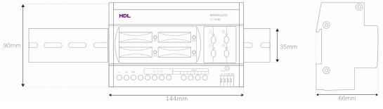
Standard 35mm Din Rail Installation
