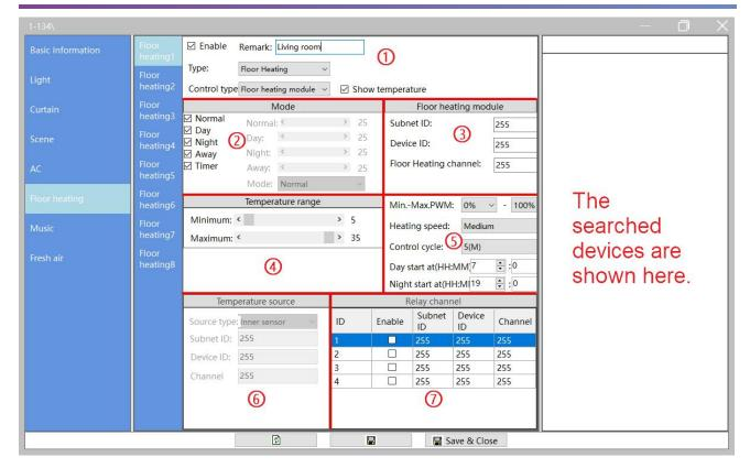
Figure 7-1 Floor Heating Setting
