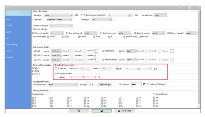
Figure 2-6 Broadcast temperature setting
