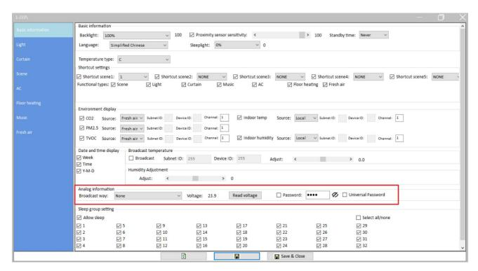
Figure 2-7 Analog information setting/read panel voltage
