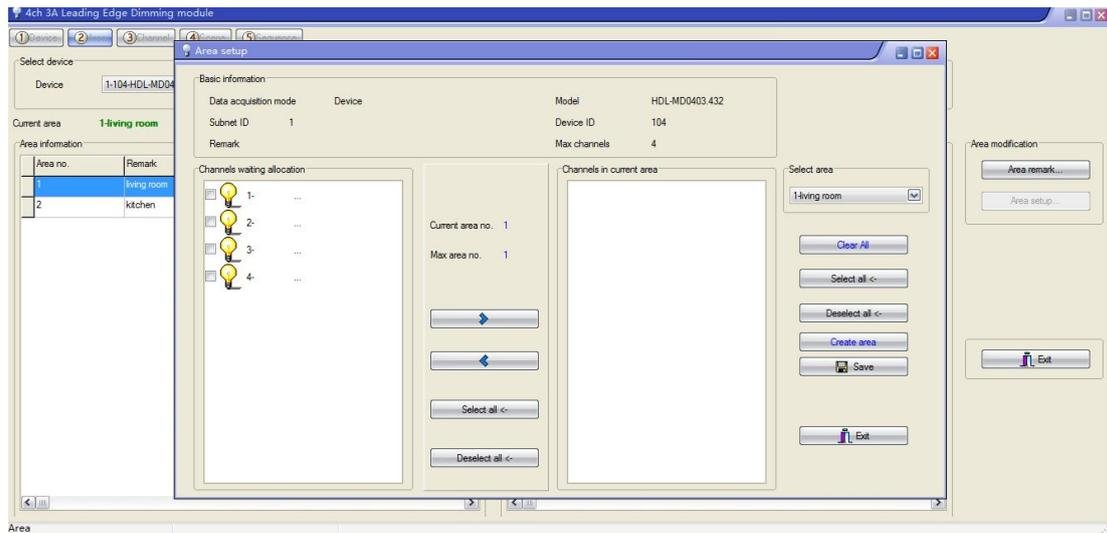
Suppose according to the wiring, channel1 to 2 are used to control 2 lights in living room, channel 3 to 4 are used to control 2 lights in the kitchen. The configuration steps would be like this:
