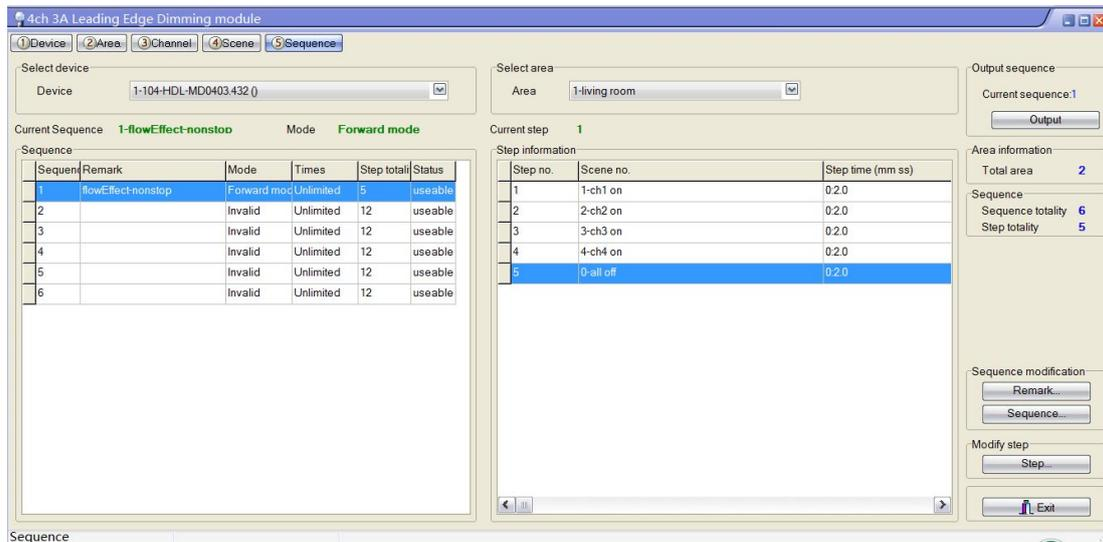
If now in area we want to create a sequence which runs this way for ever: step1 (channel 1 on) -> step 2 (channel 2 on) -> step 3 (channel 3 on) -> step 4(channel4 on) -> step 5 (channel 1, 2, 3, 4 off) -> step1 -> step2 -> step 3....
