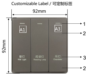
Take HDL-MP3B/Titan.48 as an example Figure 7. Dimension - Front View 图7. 尺寸图 - 正面
